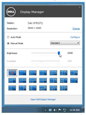
The **Quick Settings** dialog box also provides access to Dell display manager's advanced user interface, which is used to adjust basic functions, configure Auto Mode, and access other features.
